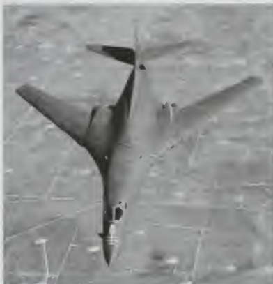
Figure 42: The B-1B, strategic bomber of the U.S. Air Force. Powered by four turbofan engines, the B-1B was designed for low-level, transonic penetration of radar defenses. The variable wings can swing forward for landing and takeoff.
